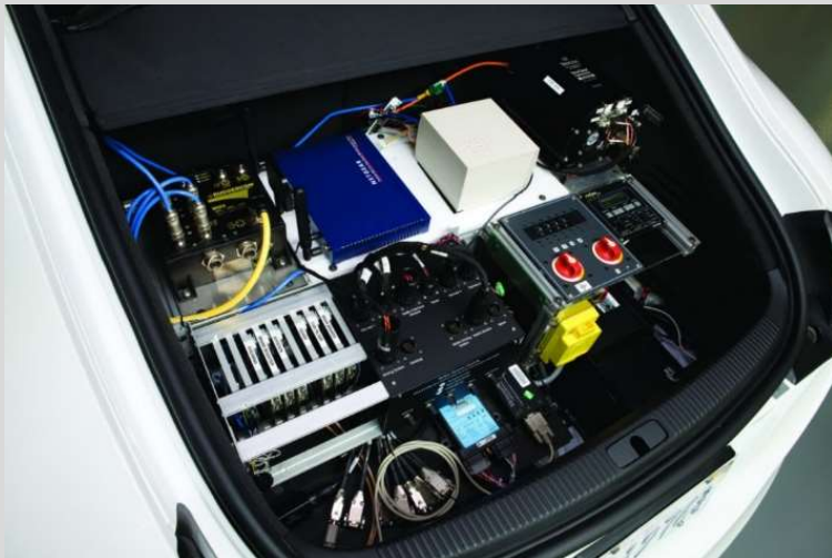
The on-board computer in Stanford's autonomous Audi TTS. (Image courtesy of Stanford University.)
