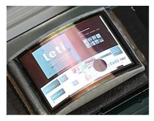
Fig. 2. Curved MICRODISPLAY CEA-LETI prototypes
